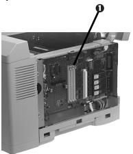
You can use these slots to add up to 64 MB of memory (two 32 MB SIMMs) to the standard 16 MB OKIPAGE 18/24DX printer memory, and/or to install either the Adobe PostScript SIMM Kit or the Flash ROM SIMM. See the Service & Support chapter for ordering information on these accessories.
