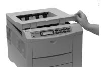
2 Lift out the used image drum cartridge with the toner installed and discard both in accordance with local regulations.
