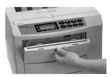
4 Flip out the manual feed tray, then pivot out the extender.
