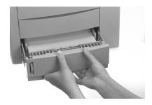
2 Remove the jammed sheet from the back of the printer.
