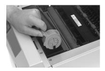
**8** Push the gray lock lever toward the back of the printer until it stops.
