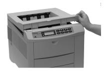
2 Pull the gray lock lever toward the front of the printer until it stops.
