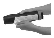
6 Place left end of the toner cartridge into the toner well at an angle, aligning the recess in the end of the toner cartridge with the tab on the image drum.
