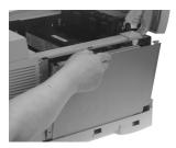
7 Remove and save the 4 screws on the left of the metal plate covering the internal board, then pull the plate out about an inch and lift it out.
