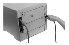
3 Detach the interface cable from the back of the printer.
