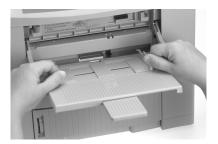
**6** Insert the envelope with return address on lower left side and flap underneath.
