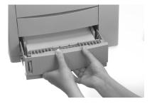
2 Reach in the front of the printer and pull the jammed sheet out of the Duplex Feeder.
