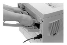
**3** *If the paper will not release*, try carefully pulling it out from inside the printer.
