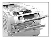
b. Swing up the paper feed cover and place the paper (up to 100 sheets) or envelopes (up to 50) on the tray. Pull out the support. Lower the paper feed cover slowly and turn the printer back on.
