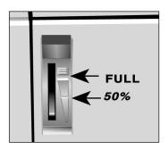
The paper tray gauge indicates the amount of paper left in the tray. This eliminates having to open the tray to check how much paper remains.
