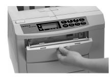
4 Flip out the tray, then pivot out the extender.
