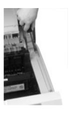
**6** Pull the side panel out and remove it from the printer.
