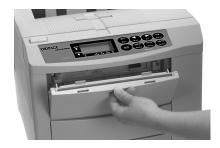
4 Flip out the tray, then pivot out the extender.
