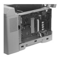
b. Insert the gold metallic contact edge of the SIMM into the socket at about a 45° angle, with the notched corner of the SIMM at the bottom. Push in until the gold contacts are fully inserted into the socket.
