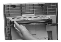
11 Locate the clear plastic film inside the front of the printer, then fold the lens cleaner over and use it to wipe any paper dust off the plastic film.
